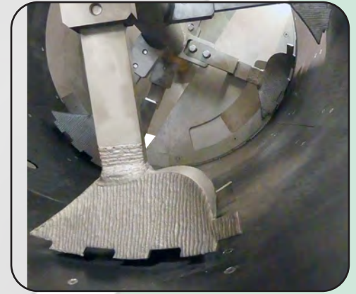
bolted, toothed ploughs in 304SS with Wolfram Carbide coating
